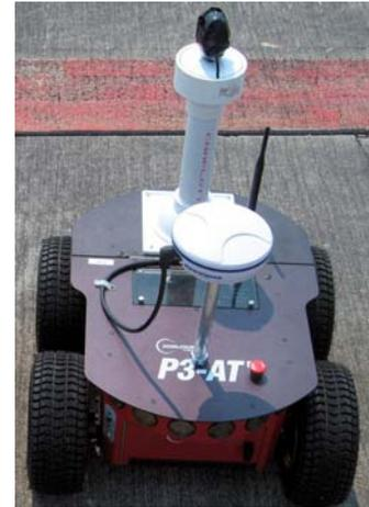
**Figure 2. Pioneer 3-AT ground robot**
