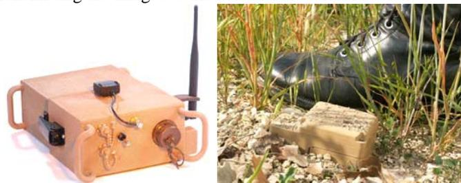
**Figure 10. Crane MicroObserver gateway and 1045 acoustic and seismic sensor**
