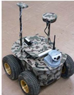
**Figure 3. Pioneer 3-AT ground robot**
